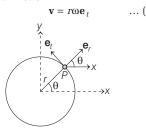
Thus, we see that velocity of the particle is  $r \omega$  along  $\mathbf{e}_t$  or in tangent direction. So, it changes as the particle rotates the circle. Acceleration of the
