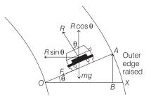
In case of friction is present between road and tyre, then Maximum speed,
